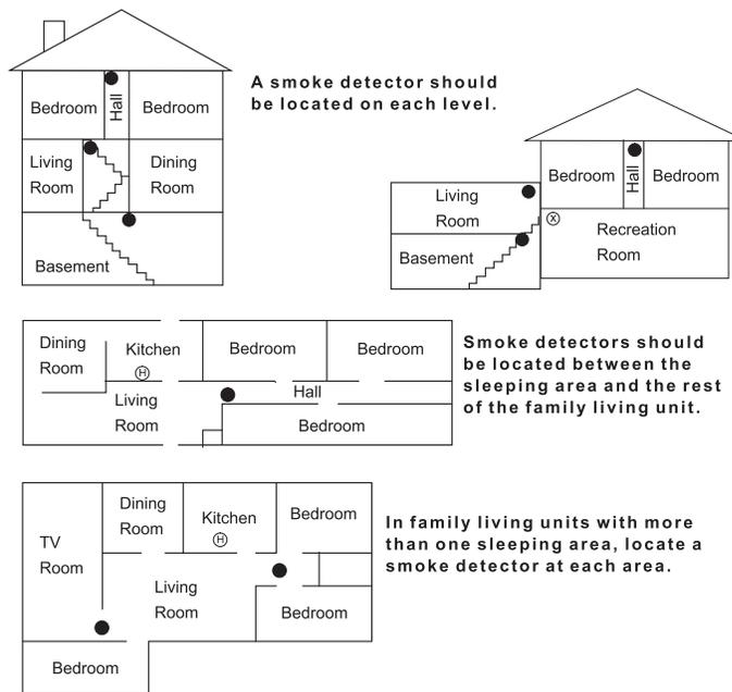
**NOTE:** Ceiling-mounted smoke detectors should be located in the center of the room or hall, or not less than 4 inches from the wall. When the detector is mounted on the wall, the top of the detector should be 4 to 12 inches from the ceiling.
